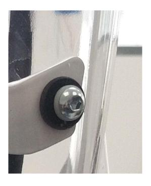
Note: Mount the plexiglas using button heads M6 screws, the nylon washer and behind the plexiglas use 5 mm neoprene washer which has an antivibration role.
