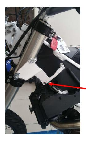
Fit the left side bracket, using initially the only screw as shown. Point the bracket in order to match the hole of the frame with the one of the bracket.
