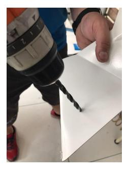
Drill holes in the side fairing, in marked points, with a final diameter 8 mm. You need to use a 5mm bit to drill this hole, then 6.5mm, finally 8mm.
